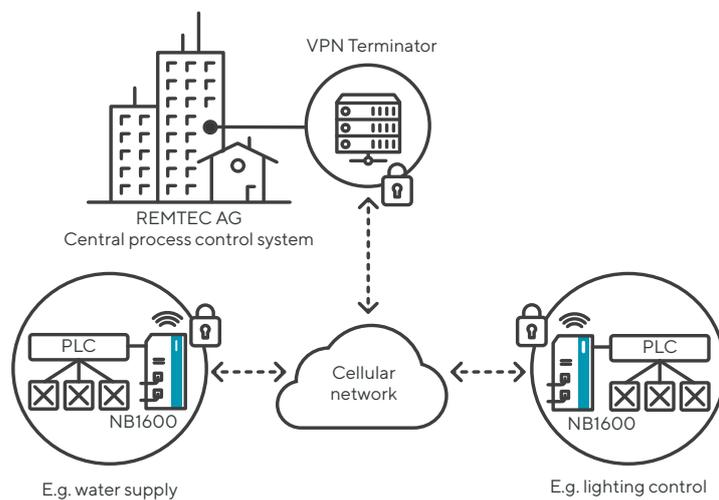
To control their actuators and sensors on site, the REMTEC AG uses a PLC which is connected via Ethernet to the NB1600. Its software supports all common VPN technologies. Thus, the NB1600 can establish an OpenVPN tunnel, which is terminated in the central process control system. Therefore, the incoming and outgoing data can be transmitted securely.
