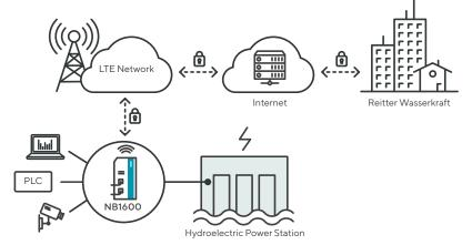
The power stations of Reitter Wasserkraft are monitored in different ways. There are in principle three possibilities: Passive queries of power, temperature or water level via a PLC in the power station, active remote access to the central computer and video surveillance. In addition to these measures, SMS messages are sent via the NB1600 in case of emergency.
