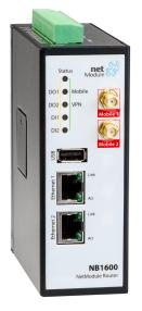
The NB1600 mobile router brings mobile broadband to the DIN rail or any other place where a fixed Internet connection is unavailable, unsuitable and too expensive.In addition all NB1600 core functions are available: digital I/O, USB and serial gateway, SDK, VPNs and many more.
