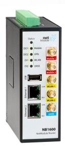
The NB1600 WIAP supports multiple wireless networks and connects them to the Internet via GSM/UMTS/LTE.In addition all NB1600 core functions are available: digital I/O, USB and serial gateway, SDK, VPNs and many more.
